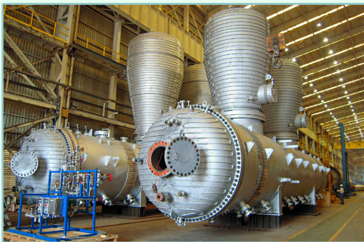
▲PP 反應槽 (PP Reactor) SA516Gr70 + SA240Tp304 φ 2,700 mm x 16,000 mm L x 112,7 Ton
