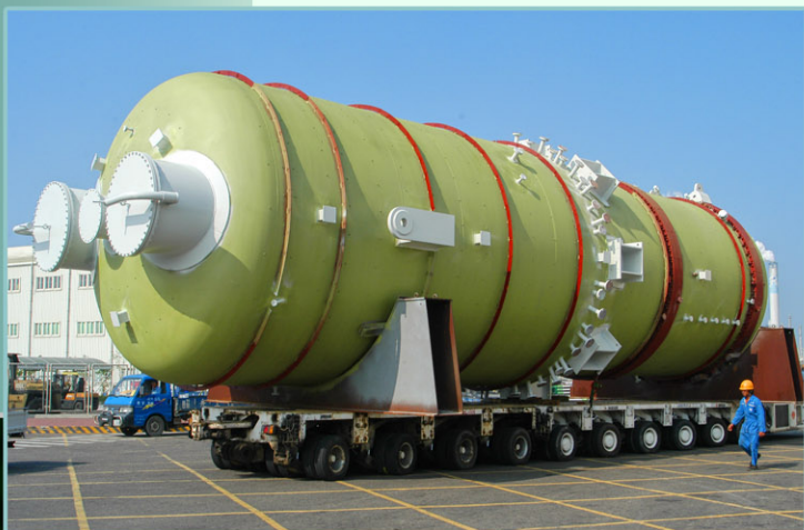
▲VCM 廠 O.C 反應槽 (O.C.Reactor for Vcm Plant) Material : Duplex Stainless Steel φ 5,000 mm x 16,426 mm L x 180 Ton
