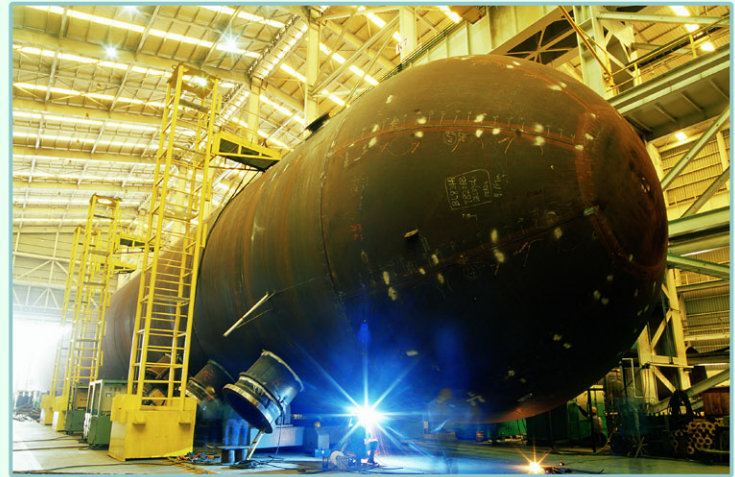
▲覆土式儲槽 (Earth Covered Tank, ECT) SA537-CI.2 \phi 7.3 m x 74.3 m L x 589 Ton
