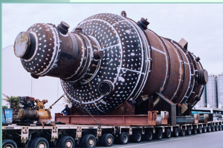
▲EO 反應槽 (EO Reactor) SA543GrB CL-1 x 117 mm T φ 7,670 mm x 22,097 mm L x 1,070 Ton
