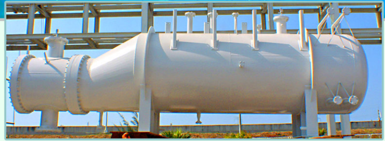
▲再生再沸器 (Dea Regenerator Reboiler) φ 2,700 mm x φ 1,525 mm x 11,318 mm L x 38 Ton Heat Transfer Area : 901 m 2
