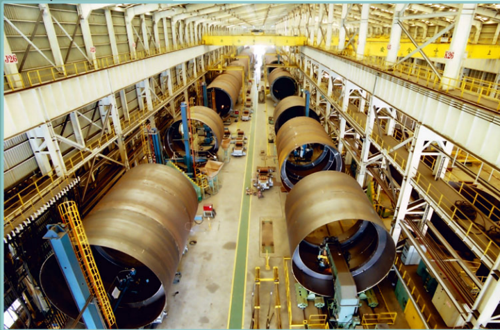
▲覆土式儲槽 (Earth Covered Tank, ECT) SA537-CI.2 \phi 7.3 m x 74.3 m L x 589 Ton
