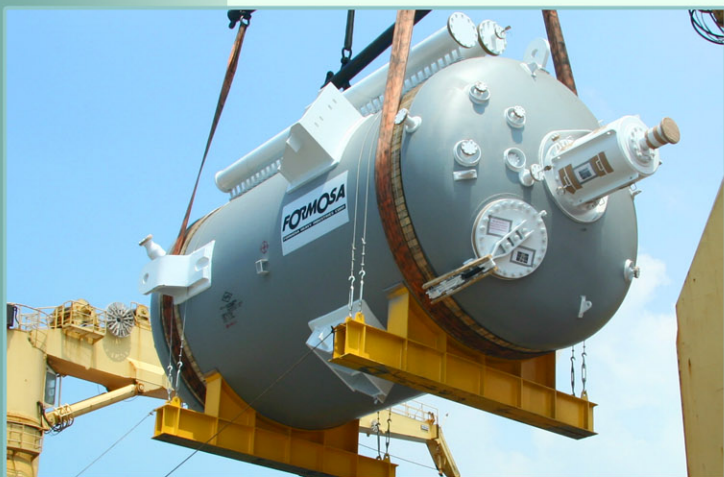
▲130 m 3 PVC 重合槽 (130 m 3 PVC Reactor) Material : Stainless Steel Clad φ 4,400 mm x 10,384 mm L x 75 Ton
