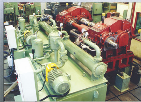
送風機用高速歯車増速機の負荷試運転 Back to Back Load Testing for Compressor Gear Increaser
